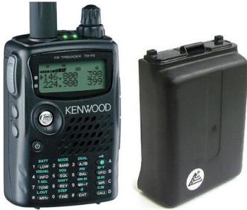
Kenwood TH-F6 (left) with standard lithium-ion battery installed. PB-42XL high-capacity battery pictured right adds 3/8”.
